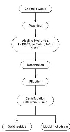
Fig. 1: The operations for obtaining polypeptide alcalin hydrolysates
